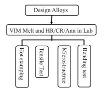
Fig.1. Schematic representation showing the experimental procedure.
