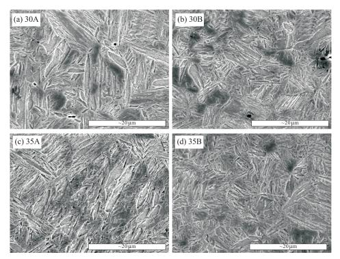
Fig.7. SEM microstructures of hot stamped alloys at 930°C, (a) 30A, (b) 30B, (c) 35A and (d) 35B.
