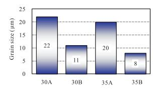
Fig.9. Grain size analysis of the four hot stamped alloys at  $930^{\circ}$ C.
