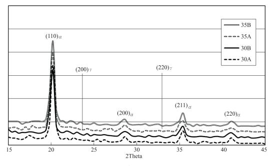
**Fig.8.** X-ray analysis of the four hot stamped alloys at 930°C.
