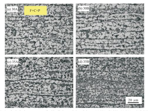
Fig.4. Optical microstructures of cold rolled annealed steel sheets, (a) 30A, (b) 30B, (c) 35A and (d) 35B.
