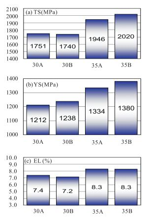
**Fig.5.** Tensile properties of cold-rolled annealed sheets after hot stamping at  $930^{\circ}$ C, (a) TS, (b) YS and (c) EL.
