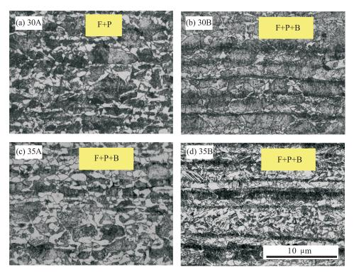
Fig.3. Optical microstructures of hot rolled steel alloys, (a) 30A, (b) 30B, (c) 35A and (d) 35B.
