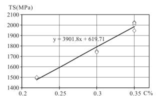
**Fig.6.** Tensile strength trend for  $0.22 \sim 0.35\%$ C MnB steels after hot stamping at 930%C.
