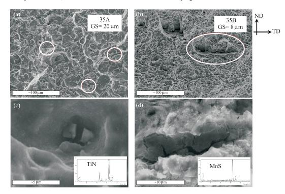
**Fig.11.** Fracture morphology of hot stamped steels after the bending test, (a) 35A, (b) 35B, (c) EDS analysis of TiN, (d) EDS analysis of MnS.
